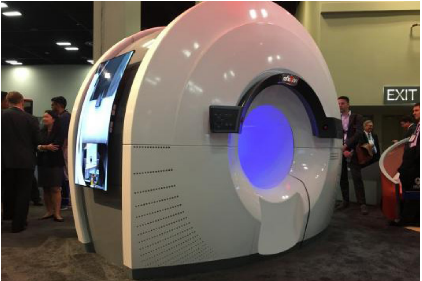
The Reflexion combination PET-CT linac, on display at ASTRO 2018. The system uses PET radiotracer emissions to track tumors directly without the need for margins to account for respiratory motion.
